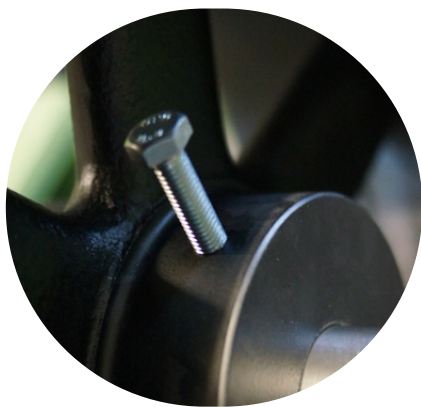
Design of the shaft-hub connection as a cylindrical bore with groove and set screw, with TaperLock bush or clamping set.
